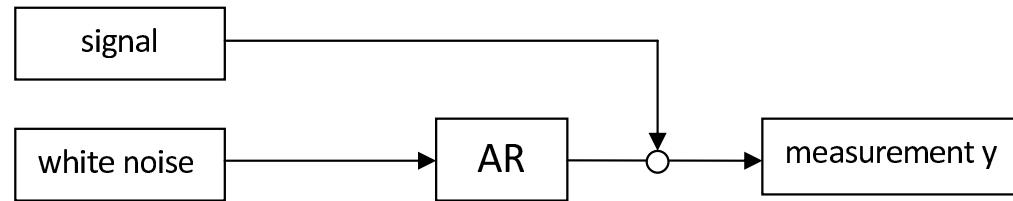
$$\text{noise} = \begin{pmatrix} 1 & -a_1 & \dots & -a_l & 0 & \dots & \dots \\ 0 & 1 & -a_1 & \dots & -a_l & 0 & \dots \\ \vdots & \ddots & \ddots & & & \ddots & \vdots \end{pmatrix} \left( \begin{bmatrix} y_k \\ y_{k+1} \\ \vdots \end{bmatrix} - Bv \right)$$
