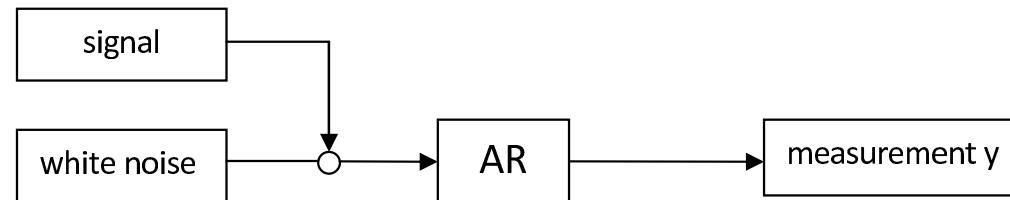
$$\begin{bmatrix} y_k \\ y_{k+1} \\ \vdots \end{bmatrix} = \begin{bmatrix} y_{k-1} & y_{k-2} & \dots & y_{k-l} \\ y_k & y_{k-1} & \dots & y_{k-l-1} \\ \vdots & \ddots & \ddots & \vdots \end{bmatrix} \begin{pmatrix} a_1 \\ a_2 \\ \vdots \\ a_l \end{pmatrix} + \begin{pmatrix} x_k \\ x_{k+1} \\ \vdots \end{pmatrix} + \text{noise}$$
