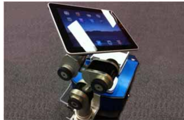
Neptune Mobile manipulator with iPad attached.
