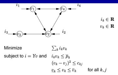
Notice:  $\overline{p}_k$  negative at loads, positive at generators. Motivation: 1) Real DC networks. 2) Approximation of AC. 3) Water tanks. 4) Supply chains
