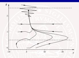
$\begin{aligned} \alpha &= 0.1, \quad \gamma = 0.1, \ \theta_0 = 1.5, \quad y_0 = 1, \quad a = 0.9, \quad \hat{\theta} = \theta_0 + \frac{a}{y_0} = 2.4 \\ y(t+1) &= (\theta_0 - \hat{\theta})y(t) + a + y_0 \\ \tilde{\theta}(t+1) &= \left(1 - \gamma \frac{y^2(t)}{\alpha + y^2(t)}\right) \tilde{\theta}(t) + \gamma \frac{ay(t)}{\alpha + y^2(t)} \end{aligned}$
